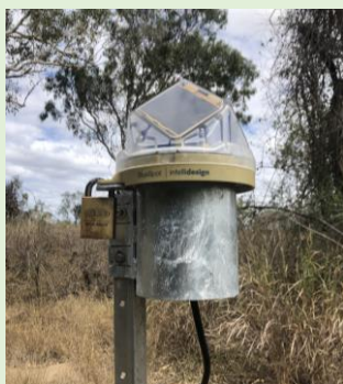
The solar head unit which powers the sensor and transmits real-time data for the Bluespot project is mounted beside the creek (left). The sensor is mounted to a galvanised steel frame and placed in the water (right).
