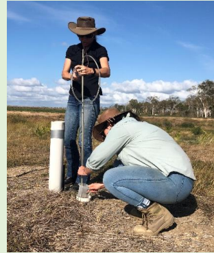
Arwen and Keeley collecting a water sample from one of the piezometers at the bioreactor for the in-situ parameter measurements.
