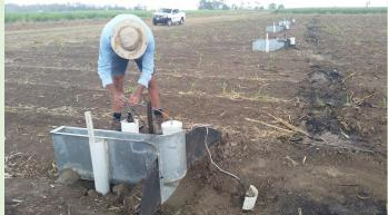
Our Technical Officer, Luke Buono, has developed a real time water quality website to be used at sites where nitrate and turbidity spectrometer equipment is installed. This gives access to fast, reliable and low-cost data and remote trouble-shooting of the equipment.
