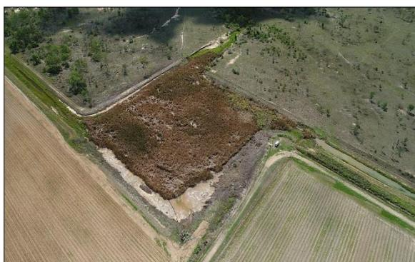
Figure 2: Project site, an old borrow pit adjacent to irrigated cane lands will be converted into a wetland treatment system.
